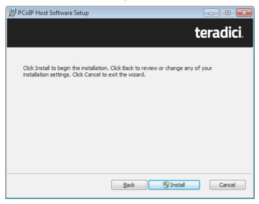
6. During the installation process, the installer might need to reboot. If so, click **OK** or **Yes** to reboot the host PC. After rebooting, the installer continues the installation.
